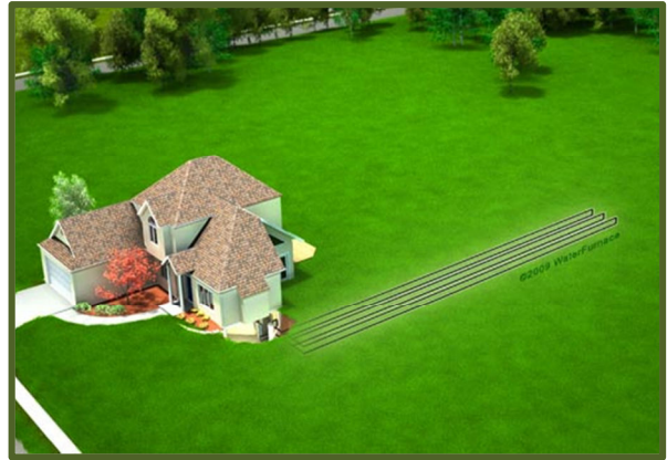
Horizontal Loop System
